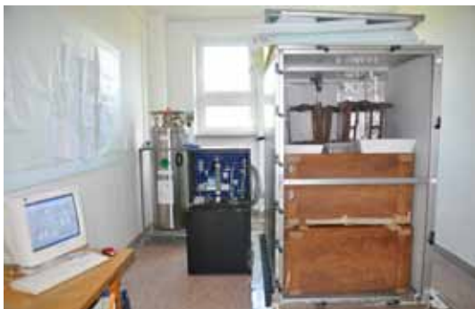
Fot. 4. Oxygenless box in progress – collection objects in the box, minitank with nitrogen, technological part of apparatus and control computer
