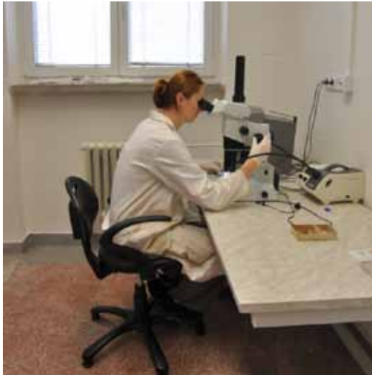
Ryc. 2. Stereomicroscope Olympus with external light source and a camera for photographic documentation of samples
