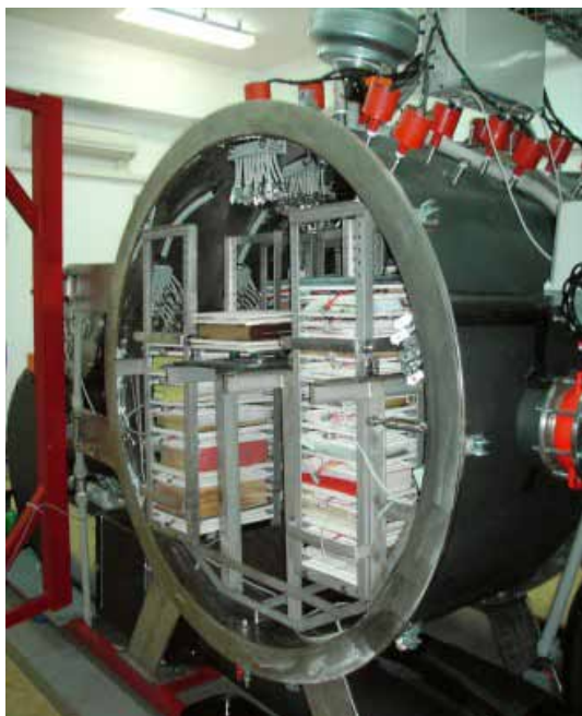
Fot. 1. Inserting books into the vacuum chamber
