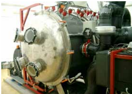
Fot. 3. Complete vacuum chamber, isolated technological part of apparatus
