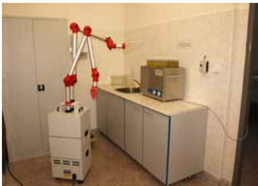
Ryc. 4. Ultrasonic cleaning machine is very useful for careful wet cleaning or as a thermostatic bath; one of the three mobile exhaust units ensure dust- and vapour-free air
