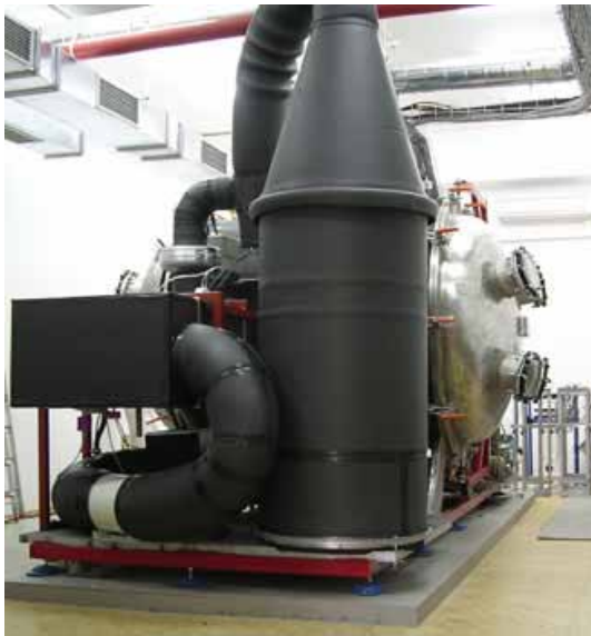
Fot. 2. Sealed vacuum chamber
