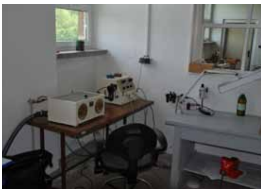
Ryc. 5. Micro sandblasting device and micro grinding machine is used for mechanical cleaning of collection objects made of metal
